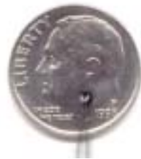
Thermox Thermistor Sensor TX-104-GB (Lake Shore Cryotronics, Inc.) 0.076mm × 7.9mm long, 7.8mg
